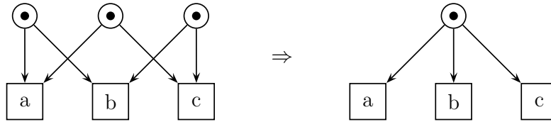
Figure 14: A distributable net which is not considered distributable in [Ho91], and its implementation.
